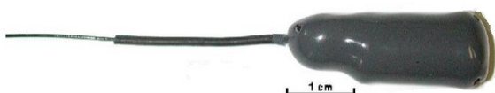
Frequency range : 138 to 235 MHz Transmitter : Crystal controlle two stage design, pulse by CMOS multivibrator
