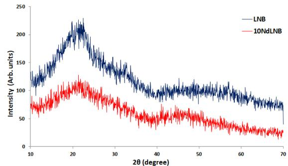
Figure 1 The XRD spectra for LNB and 10NdLNB
