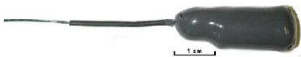
Frequency range : 138 to 235 MHz Transmitter : Crystal controlle two stage design, pulse by CMOS multivibrator pulse widyh & Rate: 20 to 24 ms, nominal 0.6 p/s (36 p/m)
